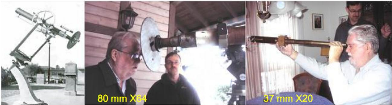
**Fig. 4.** *Left:* the 80 mm Fraunhofer refractor used since 1855 by Wolf and successors. *Center:* the same telescope in use today by Thomas Friedli (person at right). *Right:* the 37 mm portable telescope used by Wolf since the mid-1860 s.
