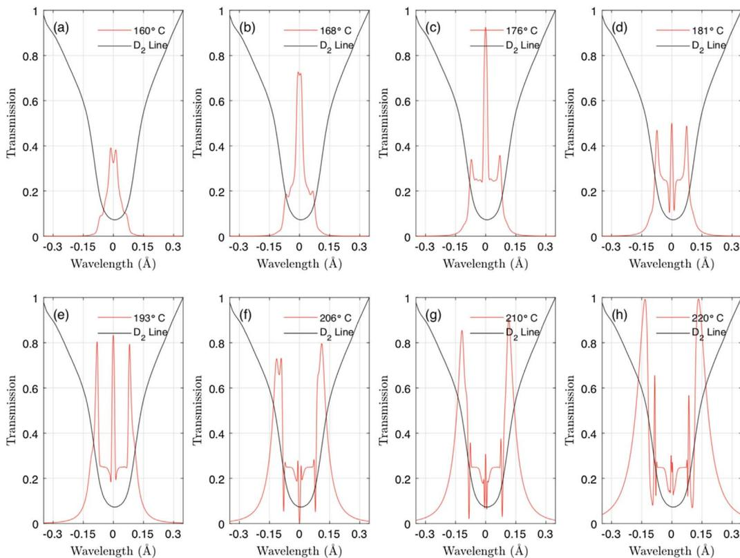
**Fig. 11.** Simulation results of transmission function for the sodium MOF. The temperature of MOF is changed from 160 °C to 220 °C. The magnetic field is 200 mT, and the length of cell is 25 mm. The Na D<sub>2</sub> line is from (Wallace et al., 2011).
