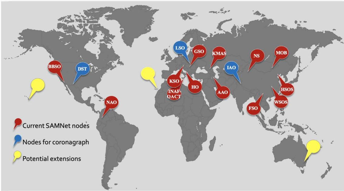
**Fig. 15.** Potential host sites for future SAMNet sentinels (see Table 2 for further facility details). The blue marks highlight sentinels with about 5–8 h time zone differences to indicate where a coronagraph could be added as 4th OTA. Yellow marks are potential future expansion sites.
